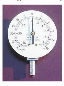
The Bourdon Gauge works a bit like the party toy that extends when you blow into it. The picture above (from Wikipedia) shows the front scale. There is a tube for connection. It measures the actual pressure. Like all instruments, it has to be standardised, but we usually buy it already standardised. As you can see from the scale, the scale is not so fine, so it only gives rough readings. These would be good enough for school experiments but not for scientists to use.
